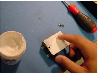
If you are truly replacing this power cube, you would want to clean old joint compound off with the same process as in Step 4.
