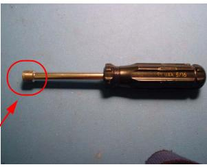
The tip of this 5/16th nut driver was ground down so that it could remove the shown nut. Without grinding down the tool, you would not be able to fit it into the power cube.
